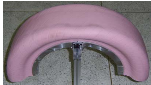
Fig. 4 Silicon mold of the air-cavity
