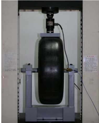
Fig. 2 Experimental apparatus for vertical loading
