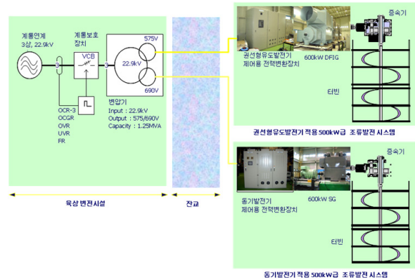
Fig. 4. Layout of the 1MW Ulodolmok Tidal Current Pilot Plant.
