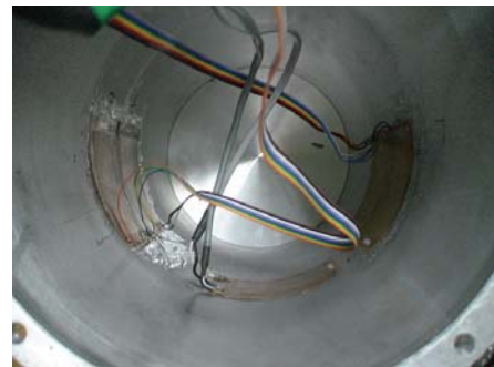
Fig. 1 Macro-composite Actuators attached to the Cylindrical Shell
