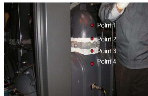
Fig. 7 Position of sound intensity probe test
