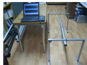
Fig. 2 FRF test of hybrid shaft
