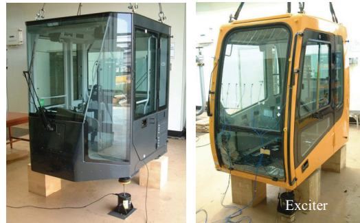
Figure 7 Experimental setup for structureborne noise
