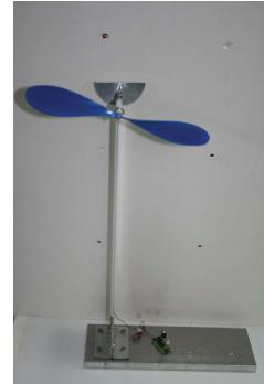
Fig. 2 Piezoelectric Energy Harvesting Device for Wind Energy
