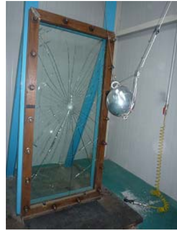
Fig. 7 Laminated glass (12.4T) after the impact (Drop height : 30 cm)
