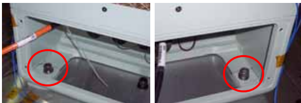
Figure1 Created crack on shock testing in console
