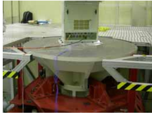
Figure7 Shock testing of console for vertical direction
