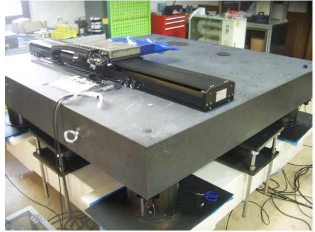
Fig. 3 Photo of a vibration control test apparatus
