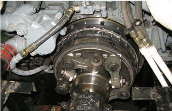
Fig. 11 Overview of Centa company's flexible coupling with flexible link
