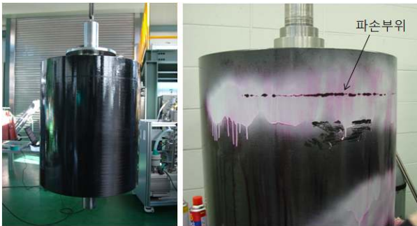
Fig. 5 Composite flywheel and torn region
