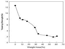
Fig. 6. Tearing strength of fabric according to weight loss
