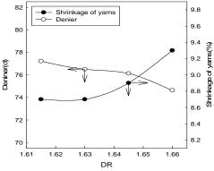
Fig. 1. Denier & shrinkage of yarn according to draw ratio
