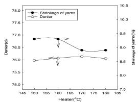
Fig. 3. Denier & shrinkage of yarn according to 1st Heater temp.
