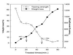
Fig. 5. Weight loss & tearing strength of fabric according to treated times
