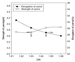
Fig. 2. Strength & Elongation of yarn according to draw ratio
