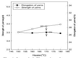
Fig. 4. Strength & Elongation of yarn according to 1st Heater temp.
