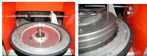
Figure 2. Spindle revolution system which consists of spindle cap and the magnetic-levitation spindle.
