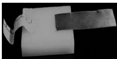
Fig.4 Adhesion of UHMPE plate to paper (left) and iron plate (right)
