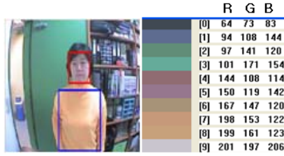
Fig. 3: 10 primary colors of the clothing area to be decided by applying the color quantization
