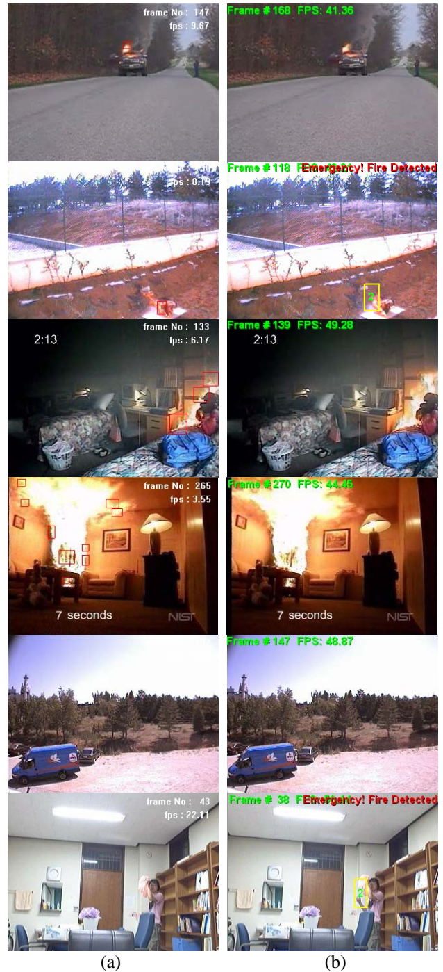
Fig. 4: Flame detection results. (a) detection results of the proposed method, (b) detection results of the Töreyn's method
