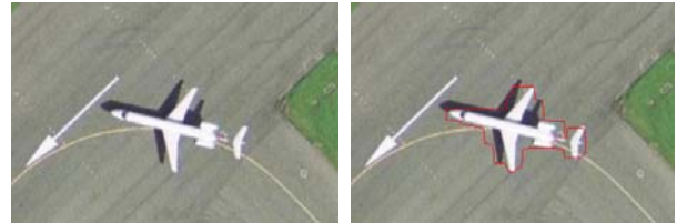
Figure 1. The object detection result from our method which use the texton histogram and object adaptive patches. The red line shows a boundary of a detected (labeled) region .
