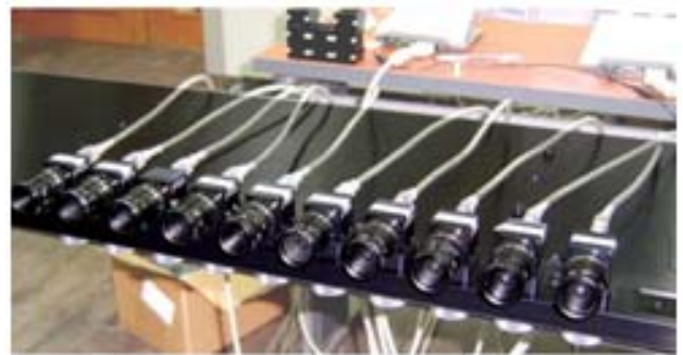
Fig. 1: The multi-view camera system which has 10 cameras in parallel array.
