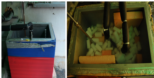
Fig. 4. Heat exchanger for low temperature air
