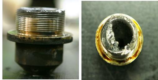
Fig. 6. Igniter after combustion test
