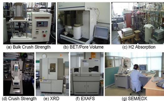
Fig. 1. Physical/Chemical Analysis Equipment
