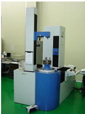
Fig. 3 3-dimensional scanner to evaluate the 2nd prototype
