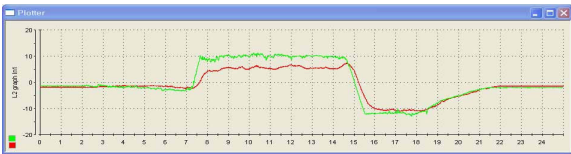
(b) Center line of the lateral displacement (green-line: leading axle, red-line: trailing axle)
