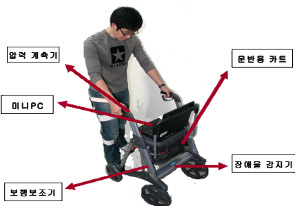
Fig. 1 Smart walker for the rehabilitation training
