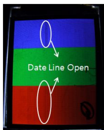
Fig. 2 Failure mode of test penal: Date line open
