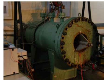
Fig. 2 Set-up for buckling test
