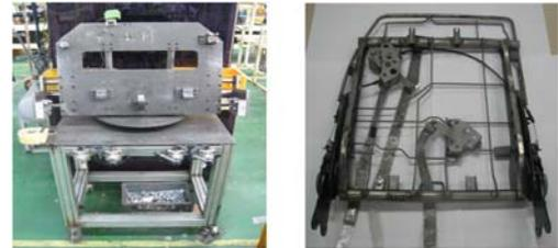
Fig. 7 Trial product of assembly jig and seat frame
