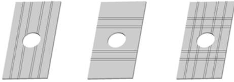
Fig. 4 A schematic of the thin plate model for hardening array (Column, Row & Cross)
