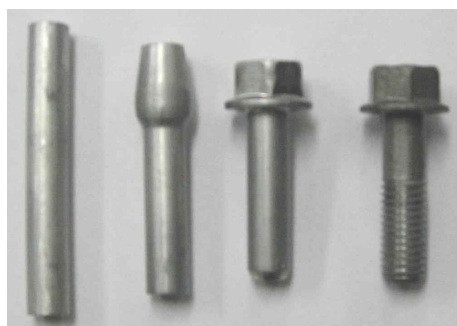
Fig. 4 Prototype of Al alloy bolt
