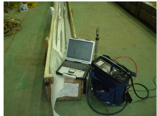
Fig. 2 System make-up of guided wave
