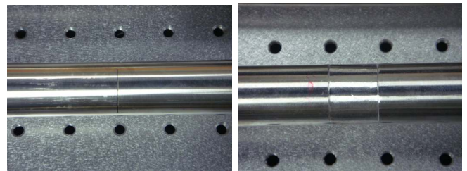
Fig. 3 Titanium tube specimen (OD 25.4mm, thickness 1.25mm)
