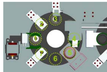
Fig.4 Layout of Turn-Table for upper part
