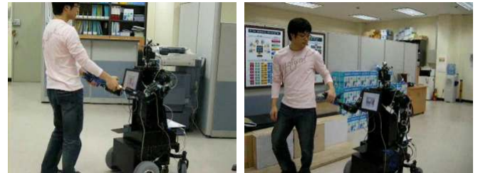
a) ambidextrous mode b) one-hand mode Fig. 5 Following human by hands
