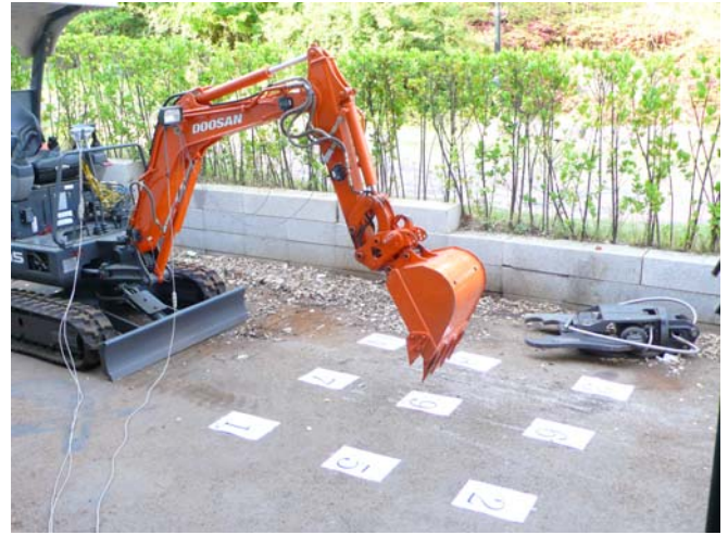
Fig. 7 Excavator operability test using haptic device
