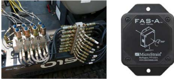
Fig. 5 Proportional valve control system and inclinometer
