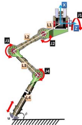
Fig. 1 A leg module for hydraulic quadruped walking robot
