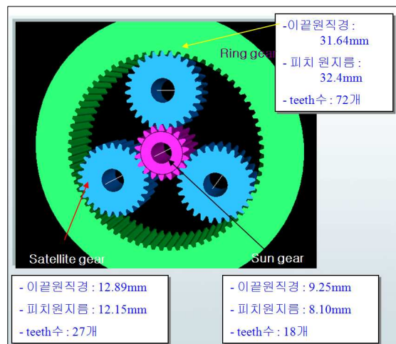
Fig.3 Gear specs dimension
