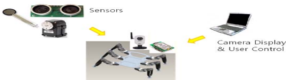
Fig.1 System configuration of the spider robot
