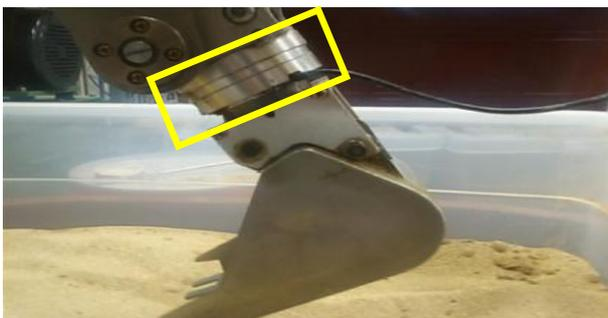
Fig. 2 Force sensor installed between bucket and arm
