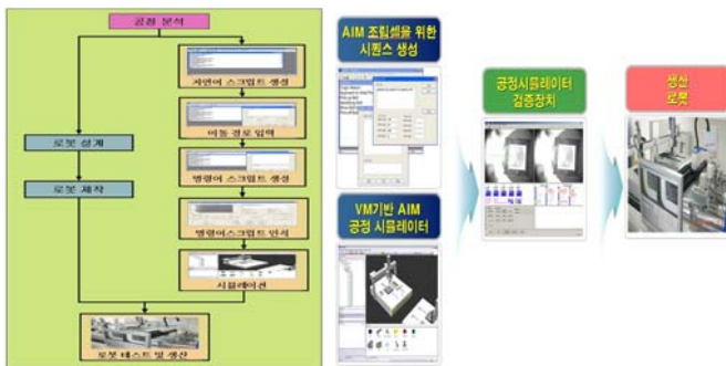
Fig. 5 Programming Process of AIM Control S/W
