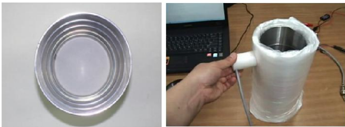
Fig. 5 Mock-up and lagging materials
