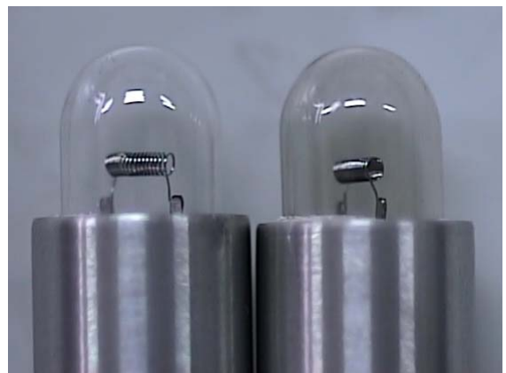
Fig. 2. Lamp bulb degradation by color center after high dose rate gamma irradiation.
