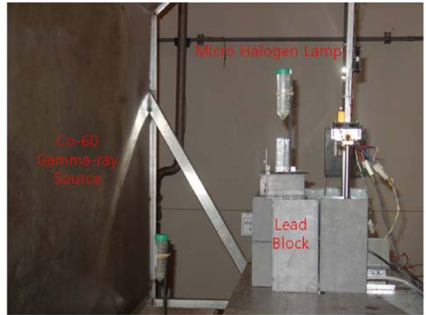
Fig. 1. Experimental setup for high dose-rate gamma irradiation of micro halogen lamp.
