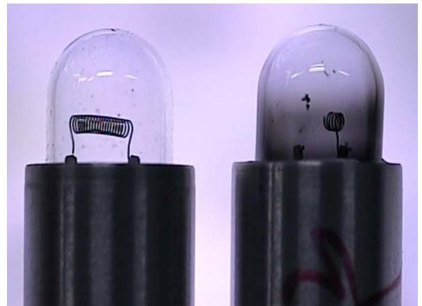
Fig. 6. Halogen lamp degradation by darkening effect (left: not irradiated, right: 8kGy irradiated )
