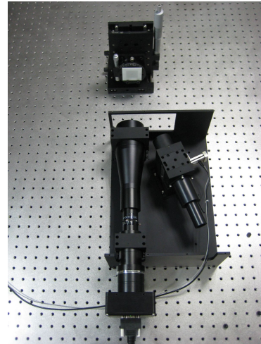
Fig. 1 Experimental setup for the measurement of optical distortion.
