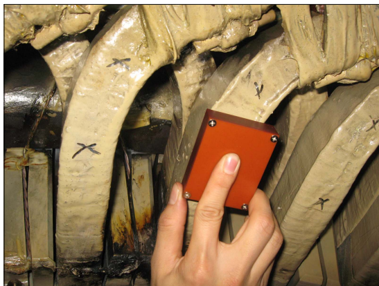
Fig. 1 Water absorption test
