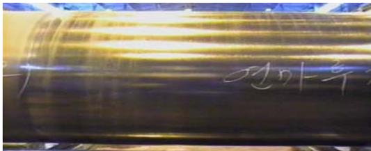
Fig 3. Typical example of fifth octave chatter marks on the barrel of a backup roll
