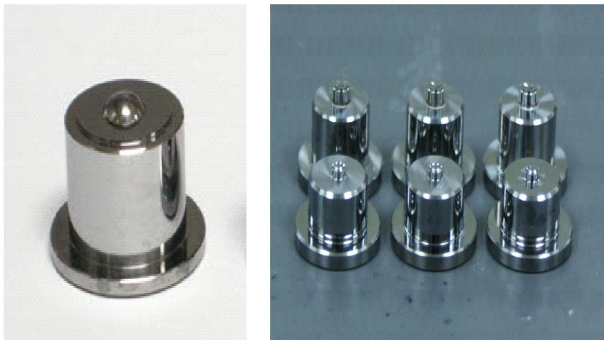
Fig. 1 Ground core with B axis minus angle alignment(-20°)
