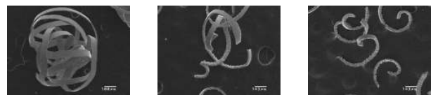
(a) cutting area 0.6mm 2 (b) cutting area 1.21mm 2 (c) cutting area 1.82mm 2 (tool width=60µm, angle=2.86°)
