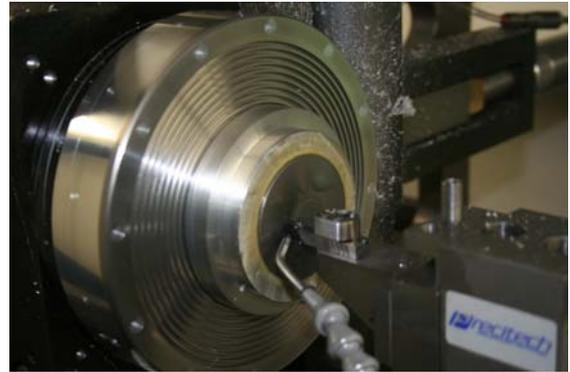
Fig. 2 The picture of ultra precision machining of Germanium
