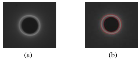
Fig. 2 Electron beam image (a) Original image(300nm, circle), (b) Edge detection image
