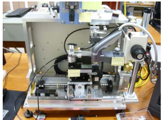
Fig. 3 Solder Ball Removing System
