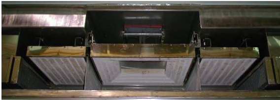
Fig. 4 Radiant heater for build room and feed room
