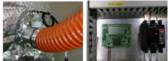
Fig. 2 Oxygen sensor and LCD monitoring board
